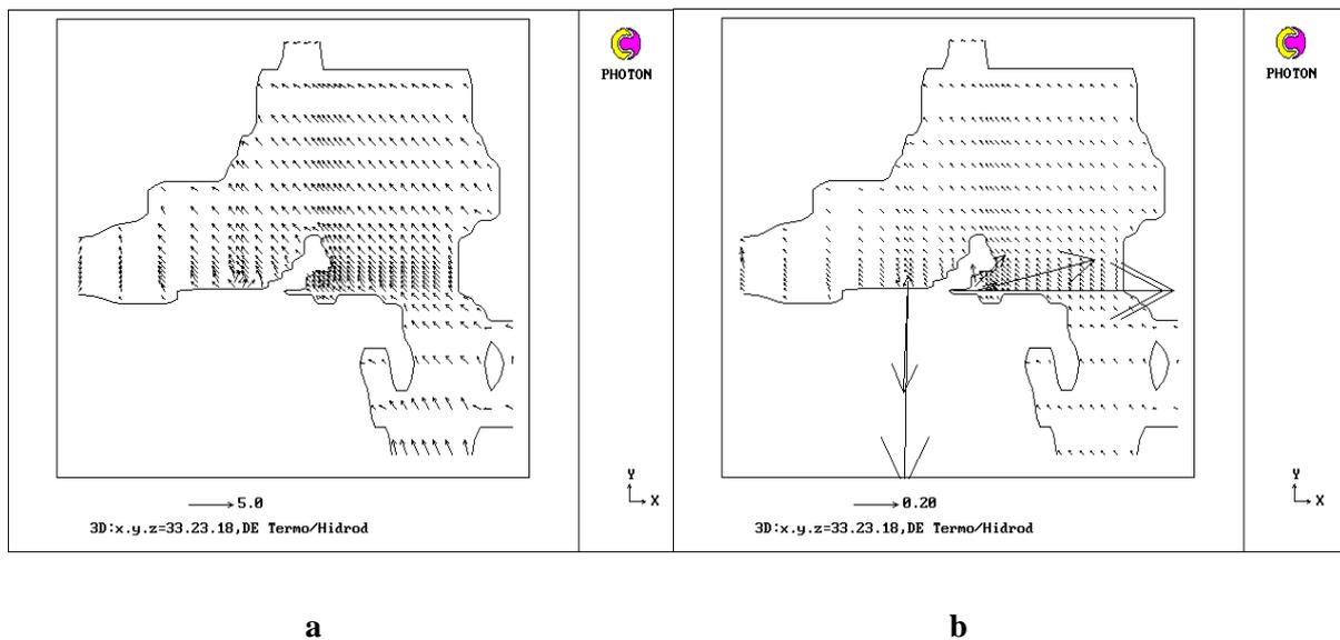
**Fig 4.** Movement of fluids at South-East mean wind velocity 1 m/s: a - horizontal vectors field in the air area 0.25 m above the water surface (vectors reference scale - 5 m/s), b - water surface velocity vectors (reference scale – 0.2 m/s)
