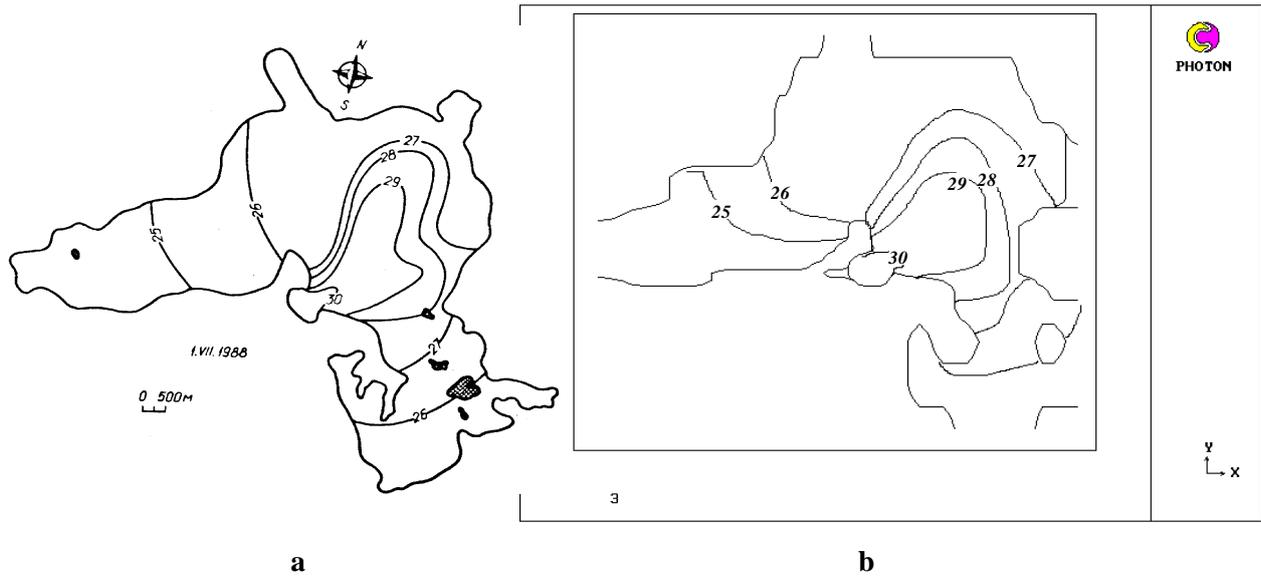
**Fig 3.** Temperature distribution on the surface of the lake Druksiai for average southeastern wind velocity of 1.0 m/s: a - measured isotherms [2], b - predicted isotherms. The air temperature is 23.9°C.
