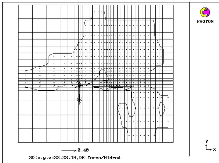
**Fig.1** Difference grid ( $x \cdot y \cdot z = 33 \times 23 \times 18$ ). The contours of the lake Druksiai with surface water velocity vectors near the inlet and outlet canals. The scale of velocity vectors is 0.40 m/s
