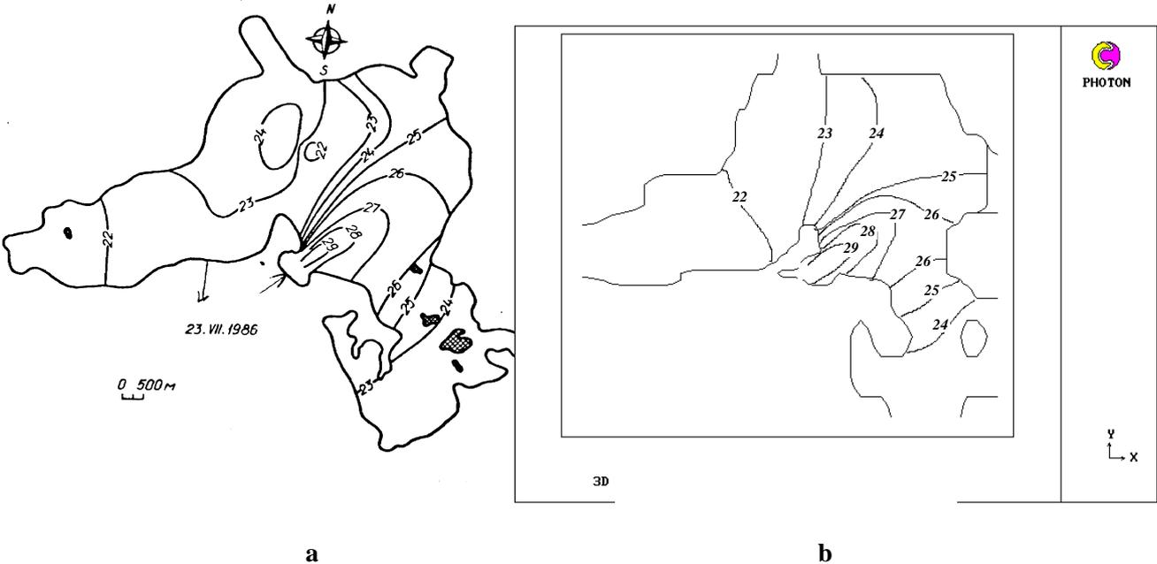
**Fig 2.** Temperature distribution on the water surface of the lake Druksiai for wind velocity - 0 m/s): a - measured isotherms [2], b - predicted isotherms
